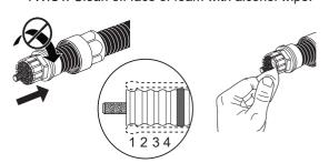
To achieve optimum Return Loss, pull outer body to remove coring bit from the tool. Place bit over inner conductor and push forward until bit contacts face of foam. BEFORE turning drill push HARD depressing foam. Maintaining force, turn drill at 1/4 trigger until tool bottoms out. Clean foam from coring bit and repeat, carefully remove any loose foam with non-metallic tool.
