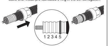
Push the collet back over the O-ring until it stops, then release it. Verify that the collet has located into the first corrugation. DO NOT TWIST. Clean off face of foam with alcohol wipe.
