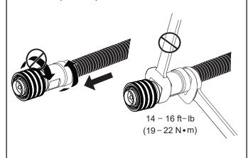
Slide the outer body over the collet and rotate slightly to align socket within the outer body with the hex edge on the collet. Push until fully engaged.
