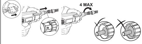
Caution: Do not apply coring/flaring bit until rear collet is in place (step 4).
