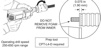
If all of the outer jacketing wasn't removed during initial cable prep remove at this time. Slide the clamping nut over the cable end. Install pre-lubricated o-ring in the 5th corrugation.
