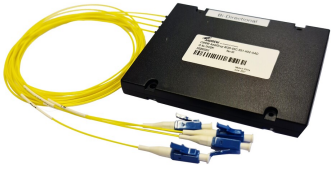
CWDM Fiber Optical Module, Add/Drop Multiplexer, 1431-1451 nm, LC/PC, 2 channels
