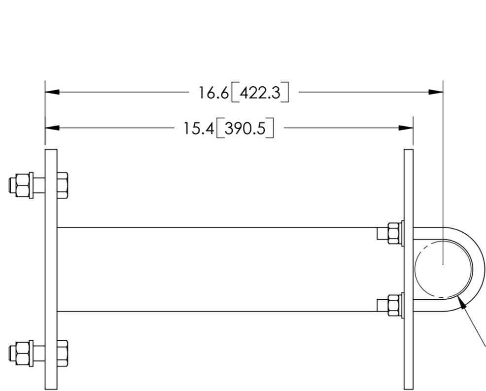
Ø 2.38" O.D. PIPES WITH INCLUDED U-BOLT
