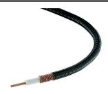
FSJ4RK-50B, HELIAX® Superflexible Foam Coaxial Cable, corrugated copper, 1/2 in, black non-halogenated, fire retardant polyolefin jacket B2ca-sla-dl-al (CPR testing is conducted annually please reference the website for latest classification)
