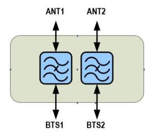
Pass Band: Tx 84-854 MHz Rx 804-809 MHz Rejection Band: 788-803 MHz Attenuation 60 dB min/ 80dB typical
